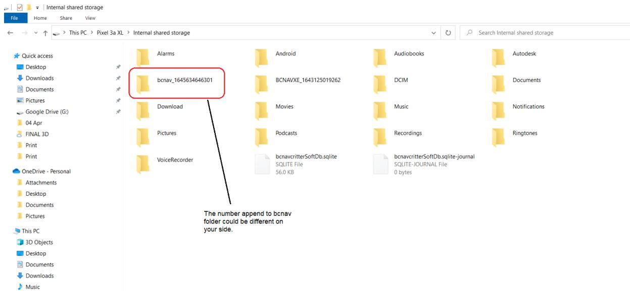
STEP 5: Paste it to the new bcnav location which is located on the following path.
